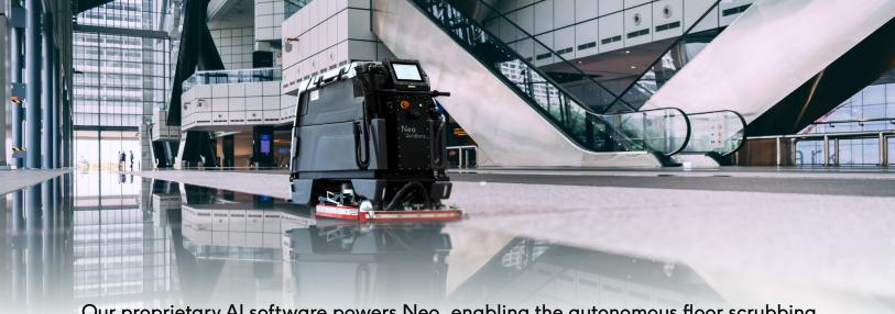
Our proprietary AI software powers Neo, enabling the autonomous floor scrubbing robot to understand its operating environment and take actions to maximize cleaning productivity while minimizing human intervention.
