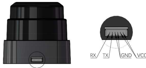
Figure 2-5 RPLIDAR S1 Female Receptacle Definition
