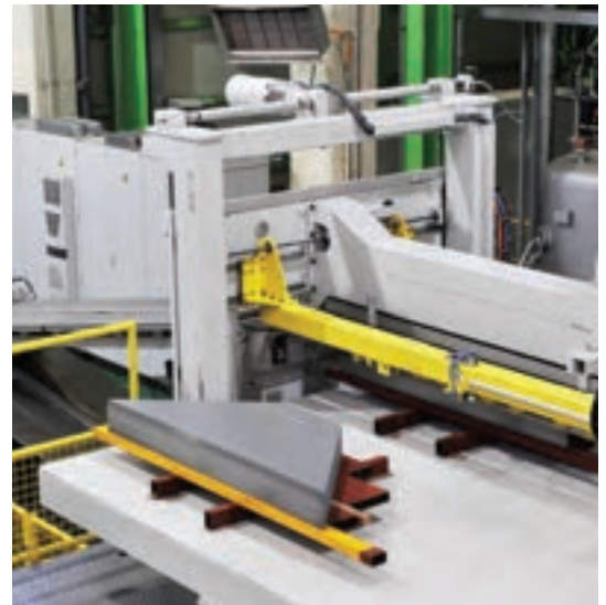
· AUTO CORE CUTTING MACHINE (CUT TO LENGTH)
