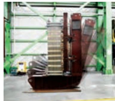
· ERECTION OF CORE ASSEMBLY
