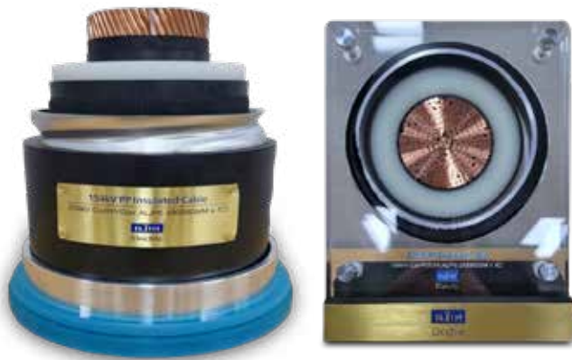
[ 154kV CU/PP/Corr.AL/PE 2500SQMM ]
